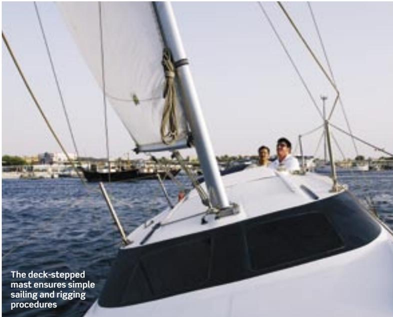
The deck-stepped mast ensures simple sailing and rigging procedures
